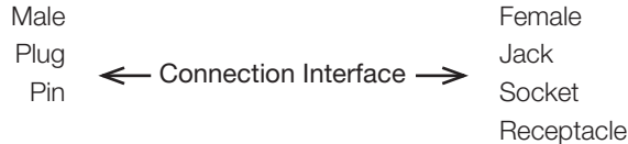
Figure 2. Typical RF Coaxial Connector Gender Terms
