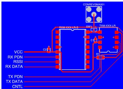
Figure 2: Example Transceiver Layout Using the LR Series
