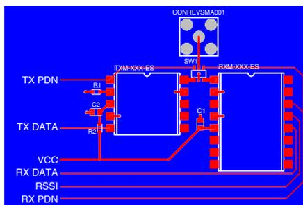
Figure 3: Example Transceiver Layout Using the ES Series
