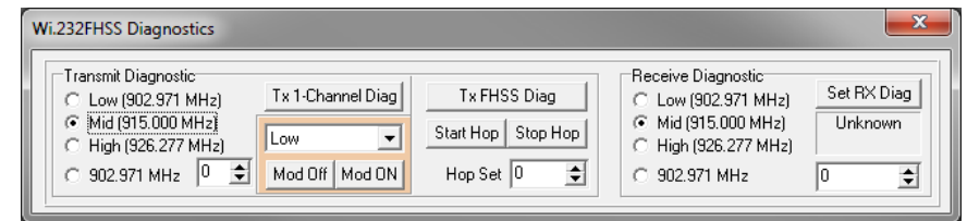
Figure 20: 250 Series Transceiver Development System Software Diagnostics Window
