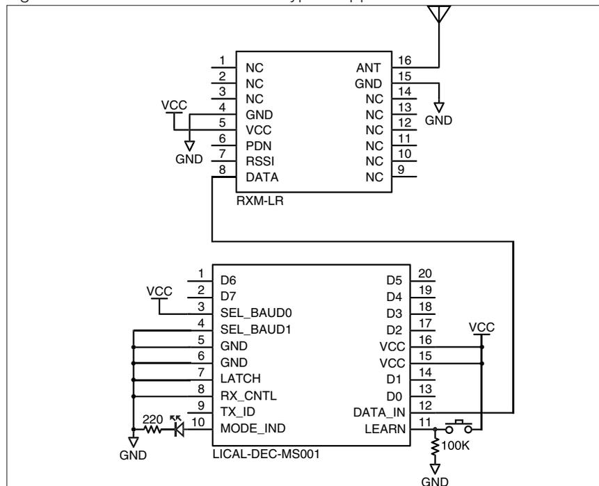
Figure 10: LR Receiver and MS Decoder Schematic
