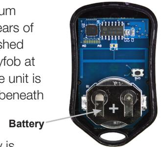
Figure 7: Battery Access
