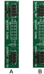
If using the USB interface, populate the USB jumpers (A) and remove the RS-232 jumpers. If using the RS-232 interface, populate the RS-232 jumpers (B) and remove the USB jumpers.
